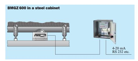
This version of the BMGZ 600 is especially suitable for tough working conditions in mobile units such as crushers and screening units.
