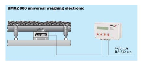
Universal electronic unit for the measurement of daily and total throughput, actual flowrate and belt speed. Various interfaces, such as RS232, analogue outputs, pulse outputs for connection of printer, remote counter or analogue meter. Ready for installation in cabinets or wall-mounting.
