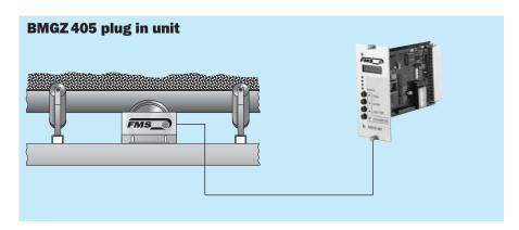
This electronic unit offers all relevant functions in an «OEM version» and was specially designed for installation in 19" systems usually communicating with a PC or an PLC. Complete remote control of the belt weigher is possible via a master system.
